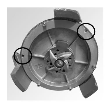
2. Install two bushings with the supplied socket head cap screws (3/16" drive).
