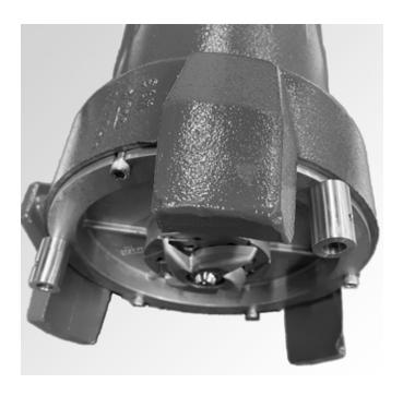
**Note**: When tightening the screw, ensure that the set screw hole is facing away from the pump centerline.
